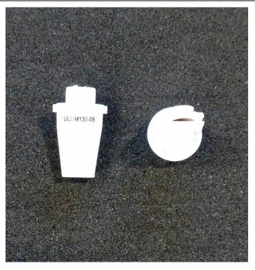
Flatfan nozzle Hypro ULDM130-08 (Plastic, white), identical to John Deere PSULDM3008
